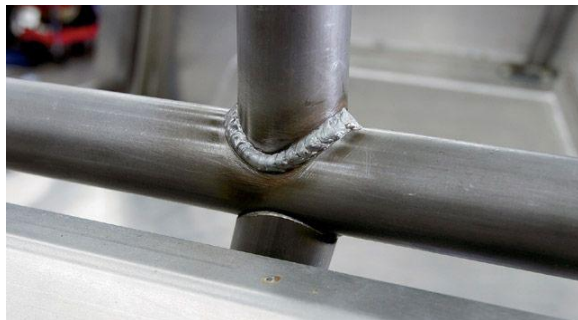
Figure 406.1.3 (2) Good Quality Weld Image
